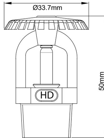
\* For T10002F/T10003F/T10004F Deflector diameter is 25 mm.
