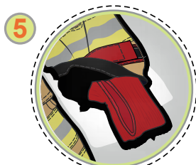
Arm end reinforcement
