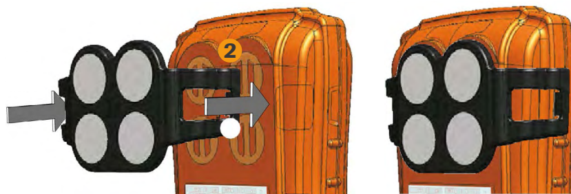
Figure 6: Fitting the external filter plate
