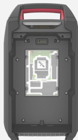
Satellite connection installed
