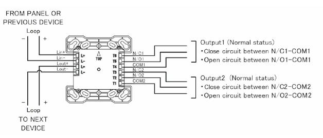
Relay Module contains two isolated sets of Form-C contacts, which operate as a DPDT switch. The module allows the control panel to switch these contacts on command. No supervision is provided for the relay contacts.
