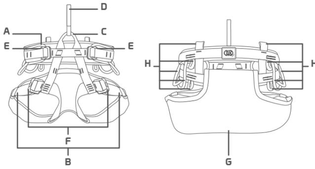
**A** Belt | **B** Leg loops | **C** Ventral attachment point | **D** Ventral attachment point (sling) | **E** Belt adjustment buckles | **F** Leg loops adjustment buckles | **G** Protective seat | **H** Gear loops
