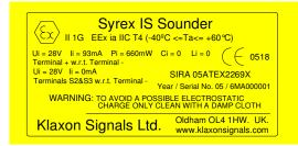
The equipment may be used in zones 0, 1 and 2 with flammable gases and vapours with apparatus groups IIA, IIB & IIC and with temperature classes T1, T2, T3 and T4.
