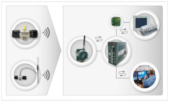
The Dräger GS01 transmits its detection signal wirelessly to the access point. From there, the signal is transferred to the gateway. This feeds the control unit directly via Modbus or with the PROFINET® protocol. For analogue analyser units, a D/A converter can alternatively be used.
