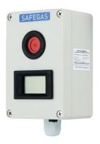
YT-96H H2 gas detector is an online monitoring fixed detector. Using imported brand electrochemical principle sensor, it's small and light, fast response, accurate detection, reliable operation and convenient for maintenance. 24V DC power supply, standard 4-20mA, RS485 signal and a set of relay signal output. It's non-explosion-proof design so need to be installed in non-explosion-proof workplaces.
