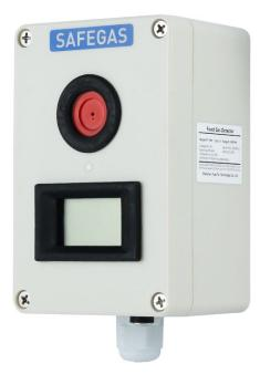
YT-96H COCL2 gas detector is an online monitoring fixed detector. Using imported brand electrochemical principle sensor, it's small and light, fast response, accurate detection, reliable operation and convenient for maintenance. 24V DC power supply, standard 4-20mA, RS485 signal and a set of relay signal output. It's non-explosion-proof design so need to be installed in non-explosion-proof workplaces.
