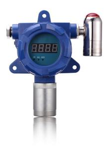
YT-95H SO2F2 Sulfuryl fluoride gas detector is a kind of monitoring gas concentration in different kinds of situations or pipelines 24h continuously wall mounted type gas detector. Using would first brand sensors, and advanced micro-process technology, with data display, fast response, high precision and good stability. Powered by 24V DC, with 4-20mA, RS485, relay signal output. Explosion proof, suitable for different kinds of situations.
