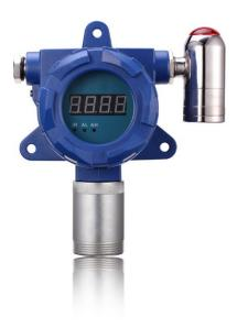
YT-95H PH3 Phosphine gas detector is a kind of monitoring gas concentration in different kinds of situations or pipelines 24h continuously wall mounted type gas detector. Using would first brand sensors, and advanced micro-process technology, with data display, fast response, high precision and good stability. Powered by 24V DC, with 4-20mA, RS485, relay signal output. Explosion proof, suitable for different kinds of situations.
