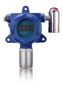
YT-95H NOX Nitrogen oxides gas detector is a kind of monitoring gas concentration in different kinds of situations or pipelines 24h continuously wall mounted type gas detector. Using would first brand sensors, and advanced micro-process technology, with data display, fast response, high precision and good stability. Powered by 24V DC, with 4-20mA, RS485, relay signal output. Explosion proof, suitable for different kinds of situations.
