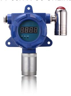
YT-95H-A O3 Ozone gas detector(with alarm light) is a kind of monitoring gas concentration in different kinds of situations or pipelines 24h continuously wall mounted type gas detector. Using world first brand sensors, and advanced micro-process technology, with data display and high/low alarm, fast response, high precision and good stability. Powered by 24V DC, with 4-20mA, RS485, relay signal output. Explosion proof, suitable for different kinds of situations.
