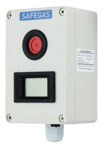
YT-96H SO2F2 gas detector is an online monitoring fixed detector. Using imported brand electrochemical principle sensor, it's small and light, fast response, accurate detection, reliable operation and convenient for maintenance. 24V DC power supply, standard 4-20mA, RS485 signal and a set of relay signal output. It's non-explosion-proof design so need to be installed in non-explosion-proof workplaces.
