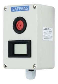
YT-96H NOx gas detector is an online monitoring fixed detector. Using imported brand electrochemical principle sensor, it's small and light, fast response, accurate detection, reliable operation and convenient for maintenance. 24V DC power supply, standard 4-20mA, RS485 signal and a set of relay signal output. It's non-explosion-proof design so need to be installed in non-explosion-proof workplaces.
