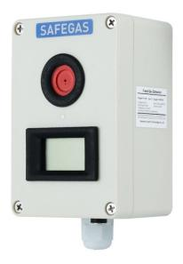
YT-96H CH3Br gas detector is an online monitoring fixed detector. Using imported brand electrochemical principle sensor, it's small and light, fast response, accurate detection, reliable operation and convenient for maintenance. 24V DC power supply, standard 4-20mA, RS485 signal and a set of relay signal output. It's non-explosion-proof design so need to be installed in non-explosion-proof workplaces.
