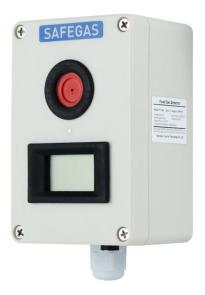
YT-96H CL2 gas detector is an online monitoring fixed detector. Using imported brand electrochemical principle sensor, it's small and light, fast response, accurate detection, reliable operation and convenient for maintenance. 24V DC power supply, standard 4-20mA, RS485 signal and a set of relay signal output. It's non-explosion-proof design so need to be installed in non-explosion-proof workplaces.
