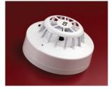
CS Heat Detector The CS heat detector (static response) uses only one thermistor and changes to alarm state at a preset temperature. Part No. 55000-137
