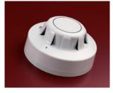
**Optical Detector** The Optical smoke detector uses a pulsing LED and a photo-diode to "see" smoke entering the chamber located within the detector housing. Part No. 55000-317
