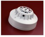
A1R Heat Detector The A1R heat detector (rate-of-rise) uses two thermistors to sense heat. Alarm state is reached when a fast increase in heat causes an imbalance between each thermistor. Part No. 55000-122
