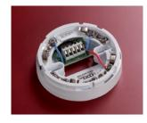
**Relay Base** The 12V relay base is designed for use in fire and security systems. For fire systems a jumper on the PCB is fitted to the 'latching' position. For security systems the jumper is moved to a non-latching position.
