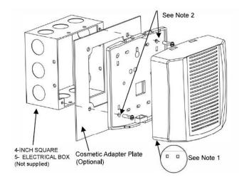
Note 1: To remove the cover, depress the snap at the bottom of the product with a key(or flat tip screwdriver) while pulling the cover up with the other hand.
