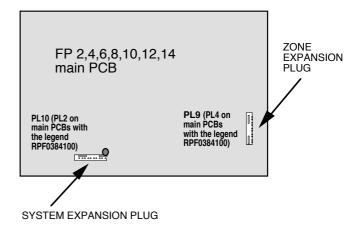
**Pinout Details:** All of these connections are very low current and MUST not be used to operate any lamps, relays etc. Note: Current drawn from these outputs will affect stand-by time.
