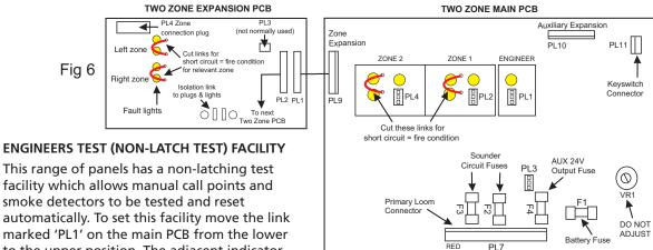
facility which allows manual call points and smoke detectors to be tested and reset automatically. To set this facility move the link marked 'PL1' on the main PCB from the lower to the upper position. The adjacent indicator will light, the warning beeper will sound and
