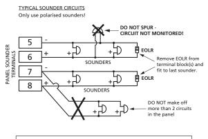
**EOLR** = End of Line Resistor ( $6k8\Omega$ , 0.25W) - supplied **CPR** = Call Point Resistor ( $470 - 680\Omega$ , 0.5W) - supplied with call point
