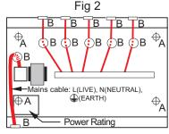
A = Mounting Holes, B = Cable Knockouts
