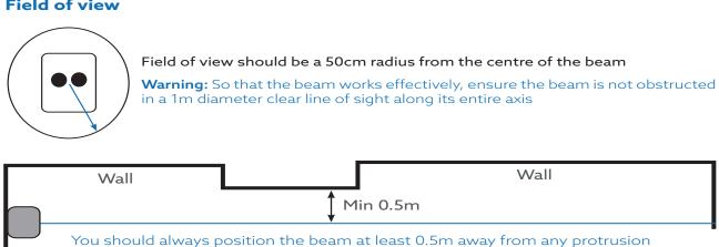
Note: Careful design consideration should be made when positioning beams and reflectors in environments that can be susceptible to condensation i.e. warehouses near to water that have areas open to the outside environment or that are exposed to quick extreme changes in temperature
