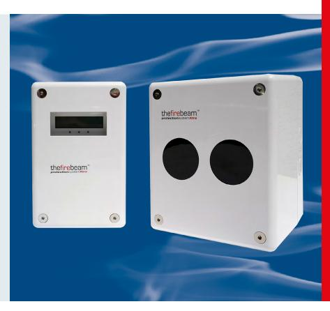
The Protec 3000/FIREBEAM/70 is a conventional beam detector, which is compatible with the Protec 3000 range. The 3000/FIREBEAM70 Reflective Optical Beam Smoke Detector includes a motorised head unit containing an infrared transmitter and receiver, a ground-level controller and prism reflector.
