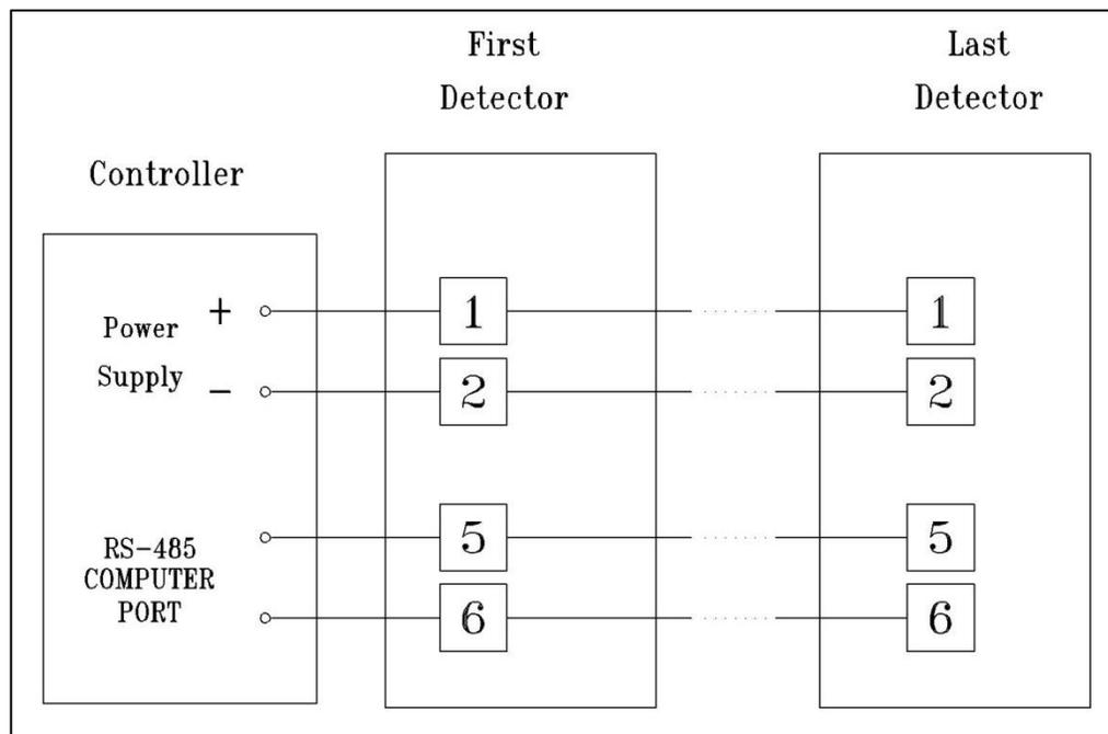
**Figure 15: RS-485 Networking for Wiring Option 3**
