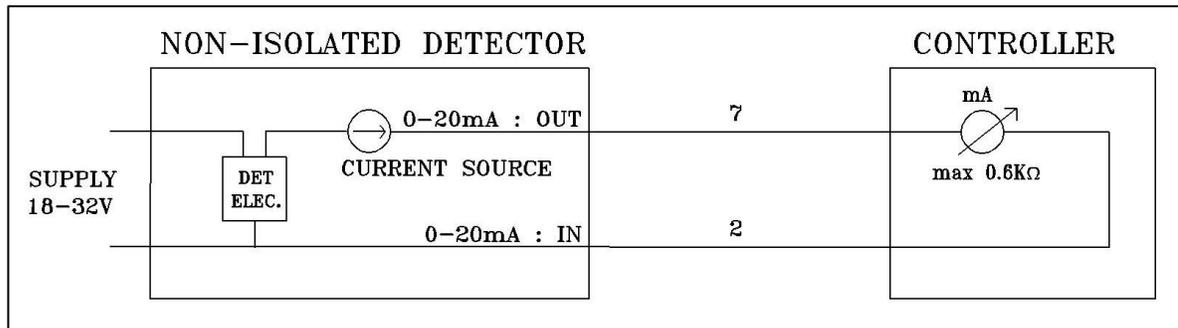
**Figure 13: 0-20mA Wiring (Source) For Wiring Options 1 and 3**
