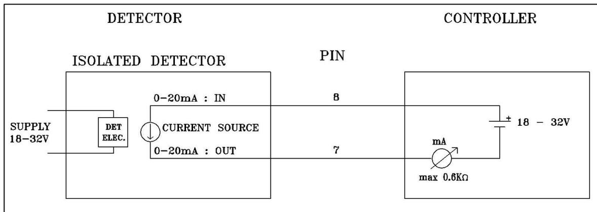
**Figure 12: 0-20mA Wiring (Sink) For Wiring Options 1 and 3**
