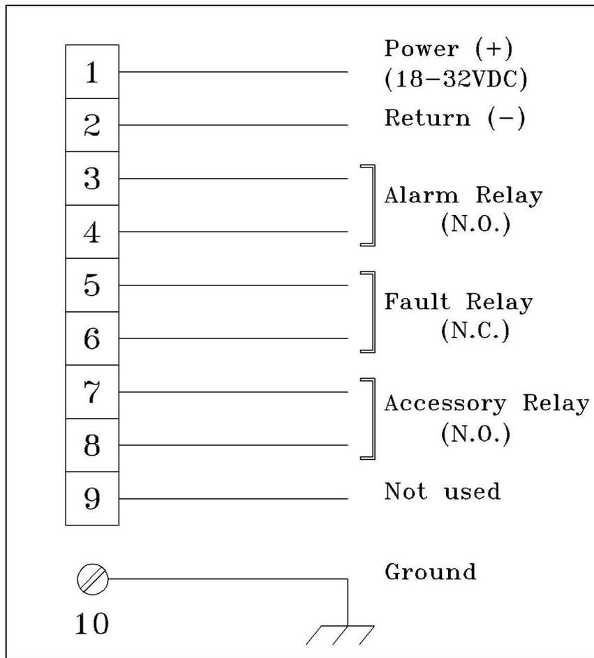
**Figure 10: Wiring Option 2**
