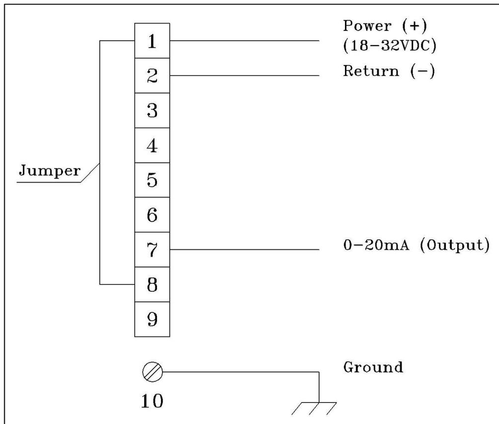
**Figure 14: 0-20mA 3 Wire Connection for Options 1 and 3**
