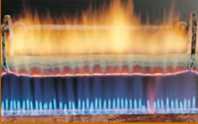
Following tests are carried out to verify if a cable is capable of maintaining circuit integrity under fire condition, fire with water, and fire with mechanical shocks. During the tests the cables are maintained at their rated voltage.
