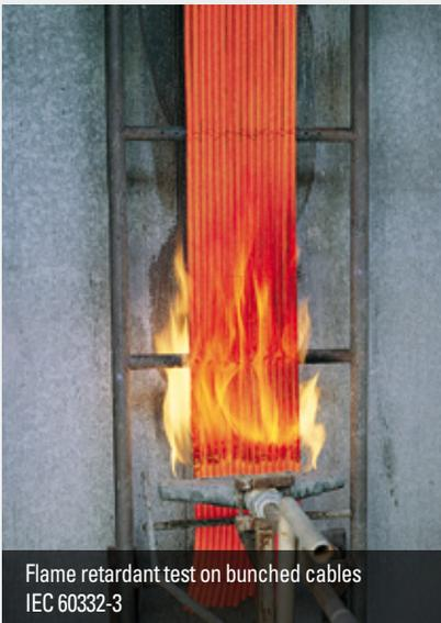
Flame retardant test on bunched cables
