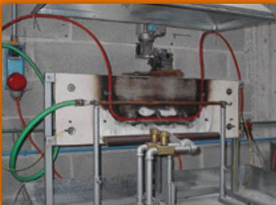
This test is carried out to verify circuit integrity during a fire. The cable is exposed to a flame at 830°C and mechanical shocks for 15 minutes and additional 15 minutes to flame, mechanical shocks and water spray. During the tests the cables are maintained at their rated voltage.
