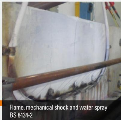
Flame, mechanical shock and water spray
