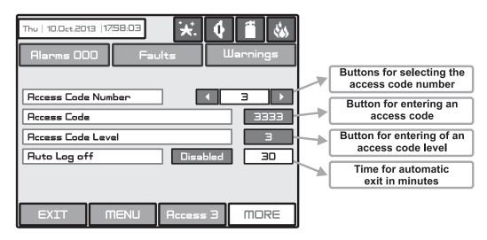
Fig. Screen 26 - Codes and Access Level Introducing.
