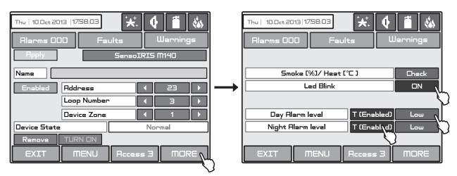
Fig. Screen 10(c) - SensolRIS M140 (IS) fire detector.
