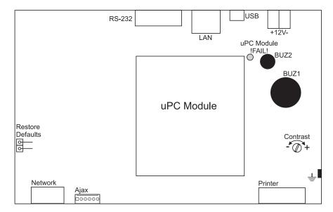
Figure 19. Main Board with integrated Control Module.
