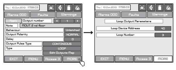
Use the button "Output Polarity" to set the type of operation of the module's relay. Every pressing of the button changes alternatively the polarity type:
