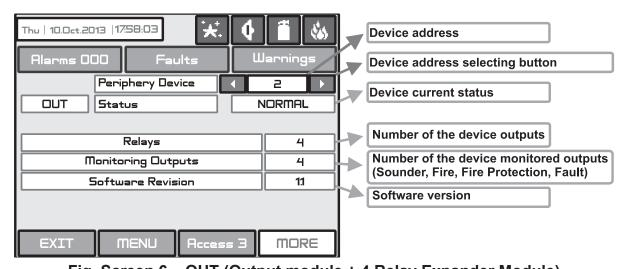
Fig. Screen 6 – OUT (Output module + 4 Relay Expander Module)
