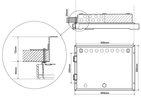
Figure 6. Mounting holes.
