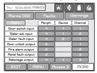
For the realization of the connection between IRIS panel and FAT/FBF panel are used *two MIO-22 modules* and *three of the programmable outputs* of IRIS panel. The MIO-22 modules are connected and addressed to the *first loop* controller.
