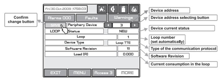
Fig. Screen 7 - Example for adding of new periphery device LOOP (IRIS TTE Loop controller)
