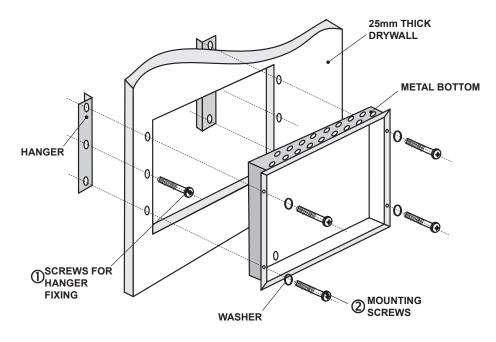
Figure 5. Action sequence for mounting.
