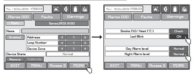
Fig. Screen 10(a) - SensolRIS S130 (IS) fire detector.
