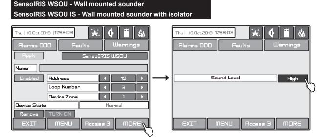
Fig. Screen 10(e) - SensolRIS WSOU (IS) wall mounted sounder.
