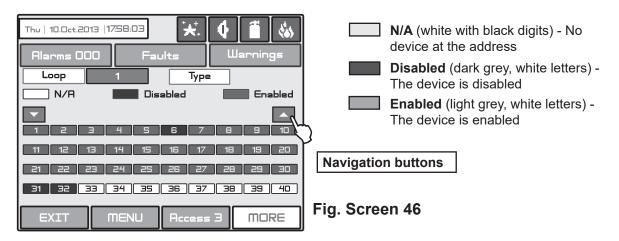
From the screen for the current status of the loop devices the user/installer can introduce new settings as choose the button with the number of the respective device 1, 2, 3...250. With the buttons ▼ ▲ is possible to be viewed the all loop devices in the system configuration. By choosing a button with a device number the user/installer moves to menu for setting of the parameters of the respective device see Fig. Screen 8, part **Programming**.
