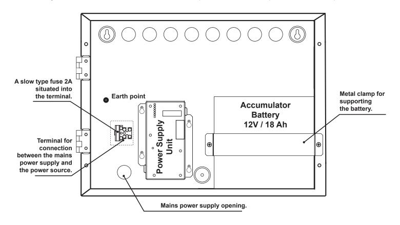
Figure 10A. Configuration of the basic modules in IRIS Repeater P and IRIS Repeater M panels.
