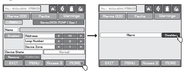
Fig. Screen 10(j) - Disabling the sounders for SensolRIS MINP (GAS).
