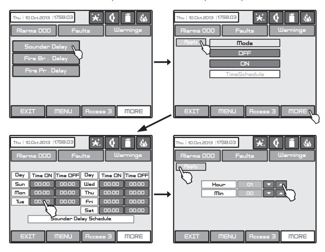
Fig. Screen 41 - Sounders Delay Introducing.
