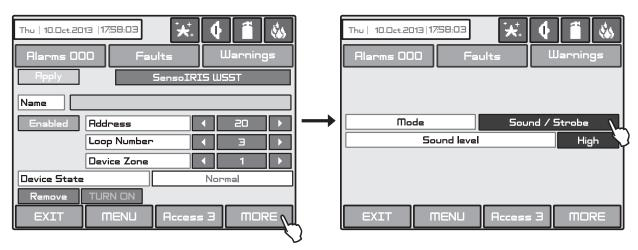
Fig. Screen 10(f) - SensolRIS WSST(IS) wall mounted sounder and strobe.
