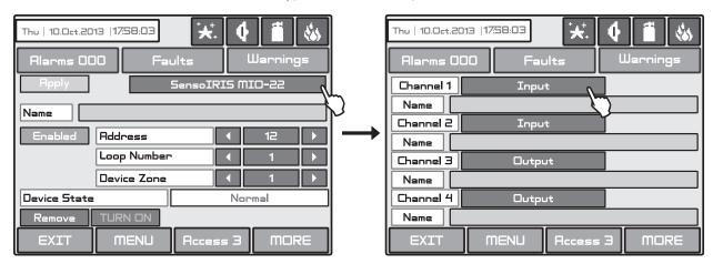
To enter the type of the event activated the input press the button next to the channel with the respective number and select one of the options. For every channel can be set a name up to 40 symbols.
