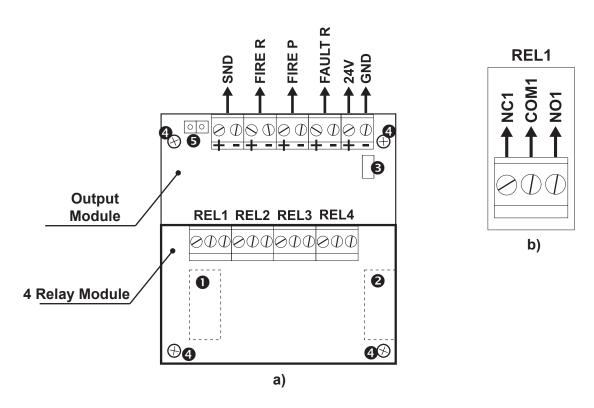
Figure 11. Output Module with integrated 4 relay module.
