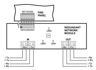
Figure 21. Connection of Redundant Network module to IRIS control panel
