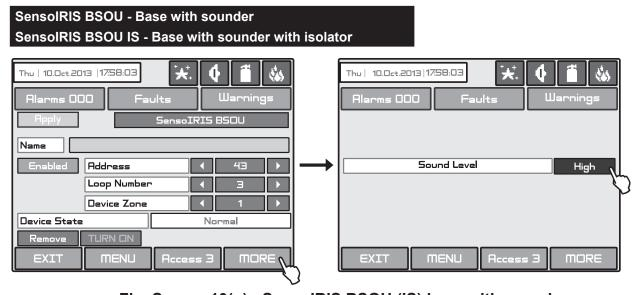
Fig. Screen 10(g) - SensolRIS BSOU (IS) base with sounder.
