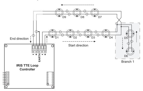
During the auto-addressing procedure the panel begins to address the devices in the loop one-by-one starting from the right positive and negative lines of IRIS TTE Loop following the direction to the right. The addresses in the possible branches on the loop continue the address numbers from the main line to the end of the branch. Then the address numbering continues on the main line and so on.
