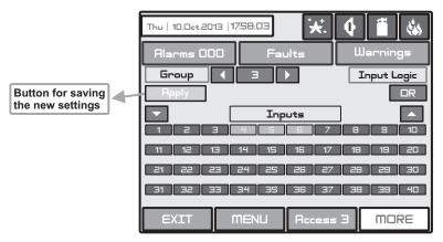
The Inputs with numbers 4, 5 and 6 are associated to Group 3 and will operate in OR logic. The OR logic function means that when any of the input is activated then the group will be activated.
