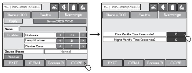
Fig. Screen 10(k) - SensolRIS MC-D fire base for conventional SensoMAG detectors.
