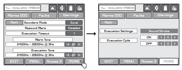
Fig. Screen 30A - Evacuation Cycle.
