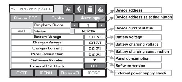
Fig. Screen 5 PSU Parameters (Power source)
