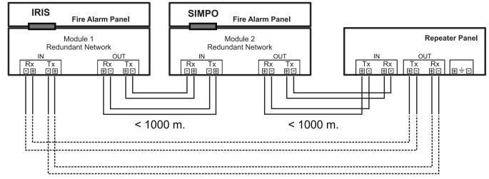
Figure 21A. Connection of Repeater panel
