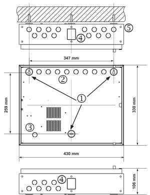
Figure 8: Elements of IRIS M (Model: PRO) enclosure
