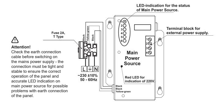
Figure 17. General view of the power source and the terminal.
