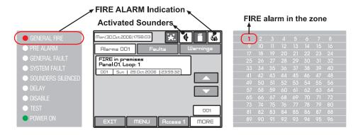
The menus for Faults, Warnings, Disablements and Tests are shown according the system status. In normal operation mode, when there are no active Disablements or Tests, only the buttons for viewing the Alarms, Faults and Warnings are displayed on the screen. If some Tests and Disablements are activated the rest of menus can be reviewed with the arrow navigation buttons.
