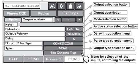
Fig. Screen 21 - Menu for introducing output parameters.
