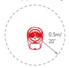
Do NOT position Detector where personnel or objects can enter the beam path Do NOT install the Detector or Reflector in environments where condensation or icing are likely to occur unless preventative measures have been taken
