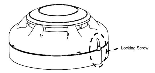
Figure 6: Position of locking screw
