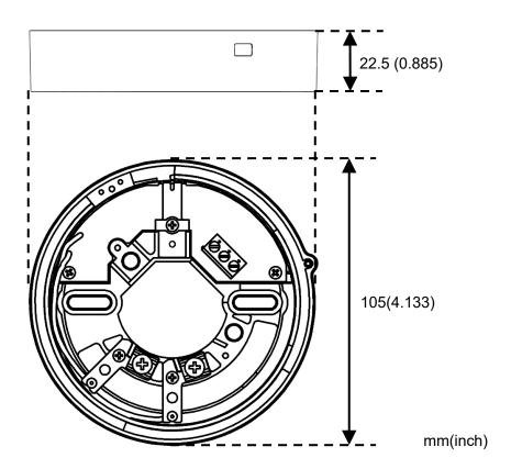
Figure 2: Dimension of VDOT-STB-RL
