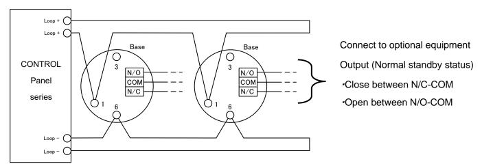
Figure 4: Connection to Zeta control panel series
