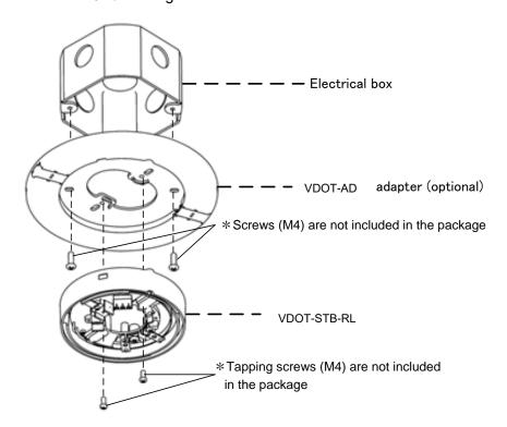
Figure 3: Installation to an electrical box
