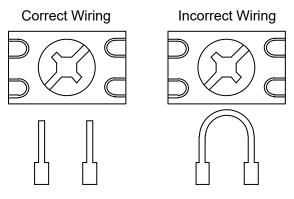
Figure 5: Connection to terminals
