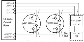
If the AUX. supply circuit needs to be monitored to detect short circuit or open circuit, connect PCE (End-of-line supervision mod-ule) to the end of the AUX. supply circuit and VDOT-MinilP to SLC.
