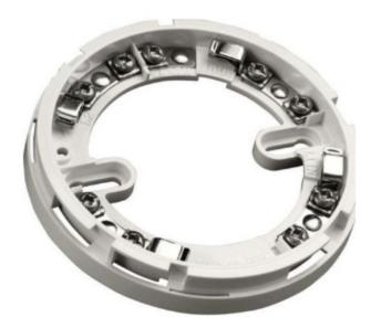
The FW Detector base has been designed for easy installation of the detector to the base, without the need of force which can be useful when mounting detectors to suspended ceilings. The detectors have a one-way fit to the base, and the FW detectors can be locked into place by a 1.5 mm hexagonal grub screw.
