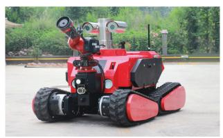
Fire robots can replace firefighters to enter the scene of hazardous disasters such as toxic, oxygen deficient, and thick smoke for firefighting, effectively solving the personal safety faced by firefighte
