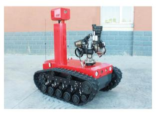
Fire robots can replace firefighters to enter the scene of hazardous disasters such as toxic, oxygen deficient, and thick smoke for firefighting, effectively solving the personal safety faced by firefighters in the aforementioned places
