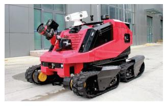
It can effectively replace trailer guns and mobile guns, and use its own power to remotely control the fire monitor or water mist fan to the desired position; Effectively replace firefighters' operations such as reconnaissance, firefighting, and smoke exhaust near fire sources and hazardous areas
