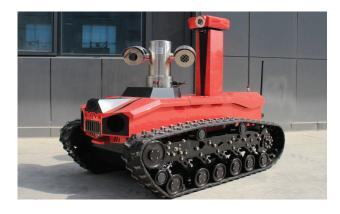
Fire robots can replace firefighters to enter the scene of hazardous disasters such as toxic, oxygen deficient, and thick smoke for firefighting, effectively solving the personal safety faced by firefighter in the aforementioned places
