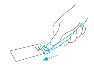
Use the small scraper at the head of the cutter for **light scraping work**: e.g. to remove labels.
