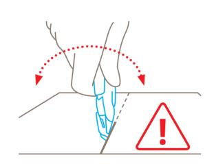
If the blade head becomes stuck, **don't force-** For best results, cut plastic strapping band fully lever the cutter!
