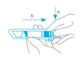
**Press** the blade change button and remove the plastic insert from the rear of the handle.
