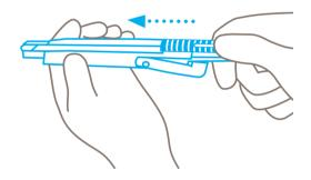
At last, slide the inner part with the blade back into the handle and flip the end of the handle upwards. Release and snap back the blade to ensure flawless functionality.
