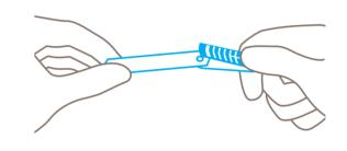
Lift the slider, take out and change the blade, then position the new blade **exactly on the cam**. For left hand use, turn blade over. The two magnets fix the blade additionally.
