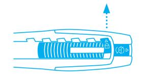
You also have the **option** of moving the slider forwards to the required cutting depth and **locking** it in position. Then **press the safety** lock into the required recess. To unlock, move in the opposite direction.
