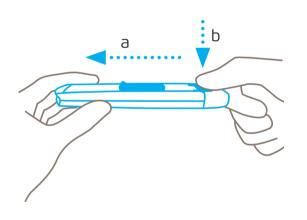
Press the blade change button **pushing up from below** and remove the plastic insert from the rear of the handle.
