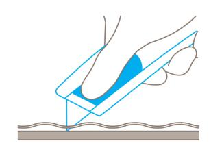
When cutting foil, be sure there is **enough counter-pressure** so that the blade does not retract by itself.
